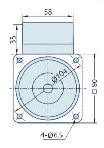
180 Watt: AC Geared Motor With Lead wires
