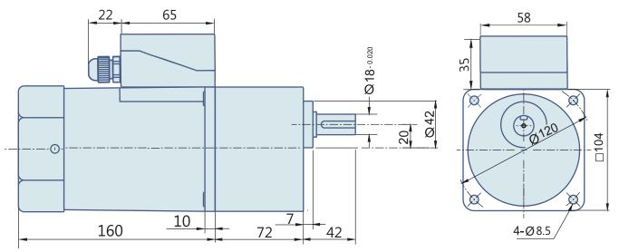
360 Watt : Round AC Induction Motor With Terminal Box
