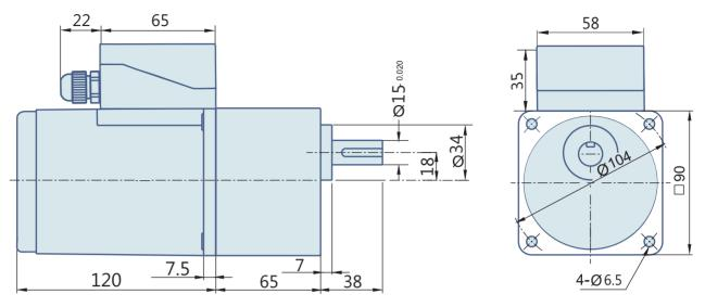
40 Watt : Round AC Induction Motor With Terminal Box
